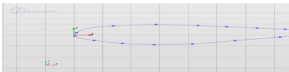
Figure 5.2 S809aero foil designing
