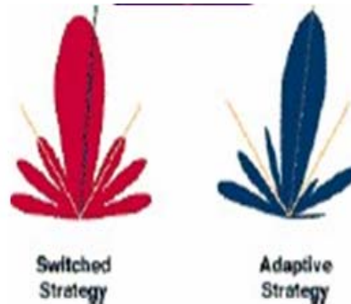
Fig.5.2: Beam forming Lobes and Nulls that Switched Beam (Red) and Adaptive Array (Blue)
