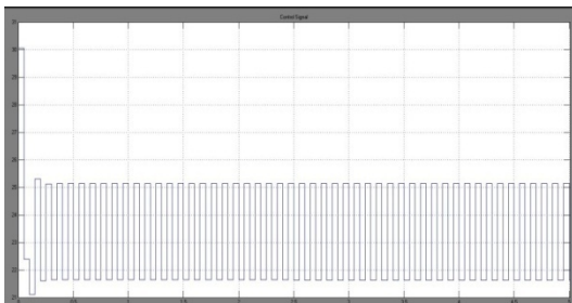
Fig. 7. Control signal (delay angle) generated by NN controller.
