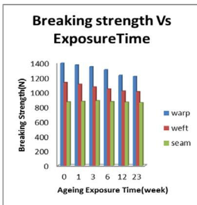
Fig. 4.2 – Breaking Strength Vs Exposure Time
