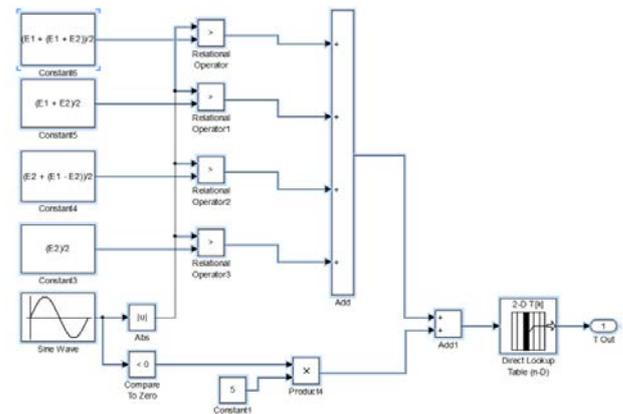
Fig.4.7- Circuit Diagram of the controller (amplitude of the sine wave is  $E_1 + E_2$ ). The Table 4.1 data is stored in Lookup Table.
