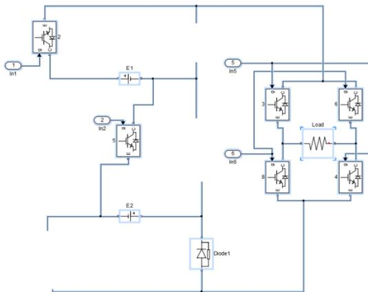
Fig.4.5- Showing the operating condition for output voltage =  $E_1 - E_2$ , only two inputs 1 and 2 are required to held in state '1'.
