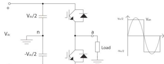
Fig.3.1 - Two-level inverter topology (left), waveform (right)
