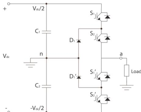
Fig.3.4- One phase leg of a three-level inverter
