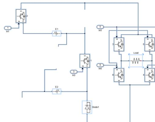
Fig.4.3- Showing the operating condition for output voltage =  $E1$ , only two inputs 1 and 3 are required to held in state '1'.
