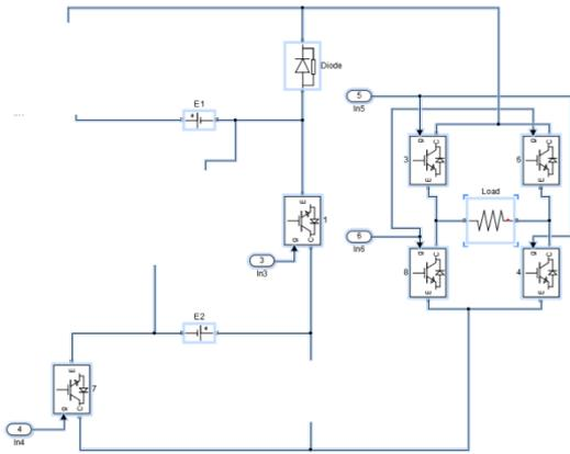
Fig.4.4- Showing the operating condition for output voltage =  $E_2$ , only two inputs 3 and 4 are required to held in state '1'.
