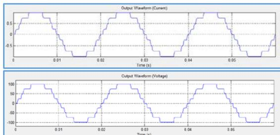
Fig.5.3- Output Voltage and Current Waveforms of inverter with resistive load.  $E1 = 75\text{Volts}$  and  $E2 = 25\text{Volts}$ , Load  $R = 100\text{ ohms}$ ,  $L = 10\text{mH}$ .
