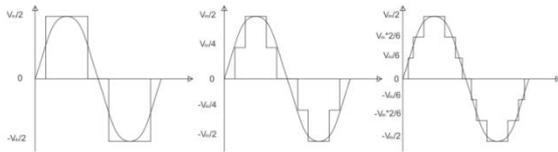
Fig.3.2- A three-level waveform, a five-level waveform and a seven-level multilevel waveform, switched at fundamental frequency.
