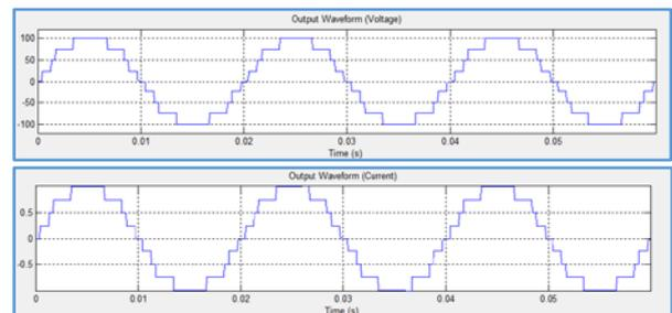
Fig.5.1- Output Voltage and Current Waveforms of inverter with resistive load.  $E_1 = 75\text{Volts}$  and  $E_2 = 25\text{Volts}$ , Load = 100 ohms.
