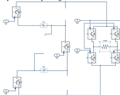
Fig.4.2- Showing the operating condition for output voltage =  $E1 + E2$ , the three inputs 1, 3 and 4 are required to held in state '1'.
