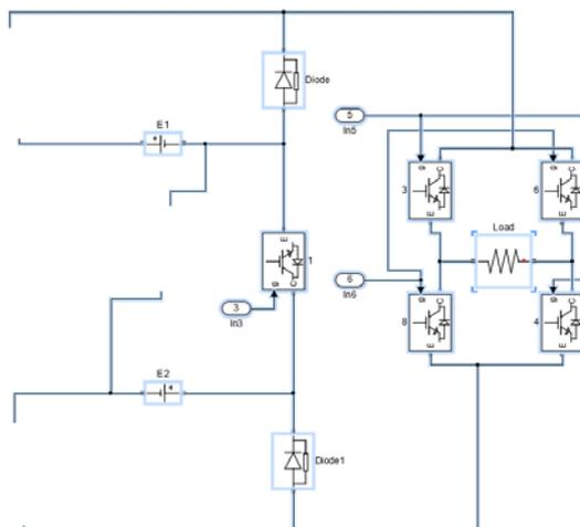
Fig.4.6- Showing the operating condition for output voltage = 0, only two inputs 1 is required to held in state '1'.
