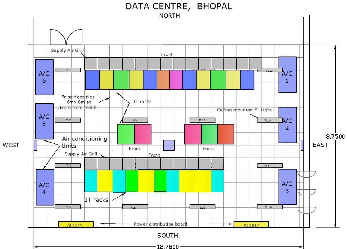
Fig. 5.1- Floor plan of showing equipments
