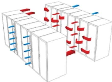
Fig. 1.2- Floor-mounted row-based cooling [3]
