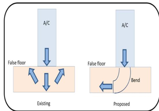
Fig. 5.2: Provision of bend at A/C discharge outlet
