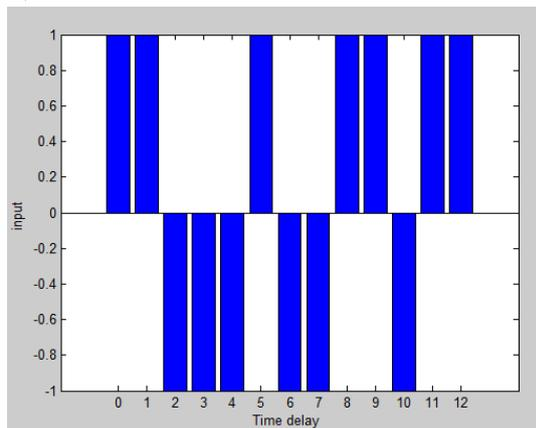
Fig. 3.2 - Representation of input barker code.
