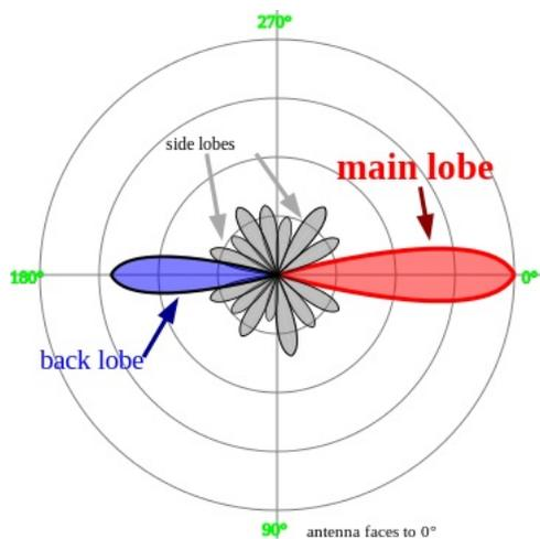
Fig. 3.1 – Horizontal Antenna Pattern
