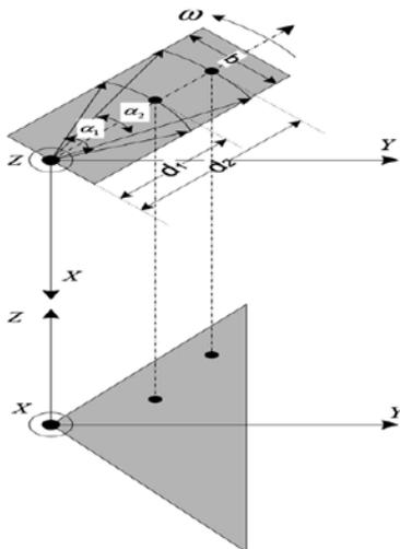
Fig. 4.1 - The lighthouse approach for distance measurement
