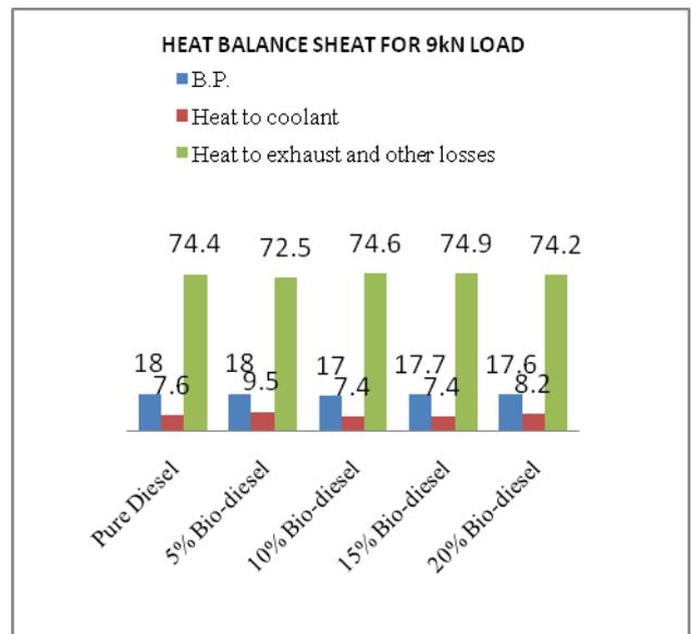
Fig. 7.6 Heat balance sheet for 9 kN Load
