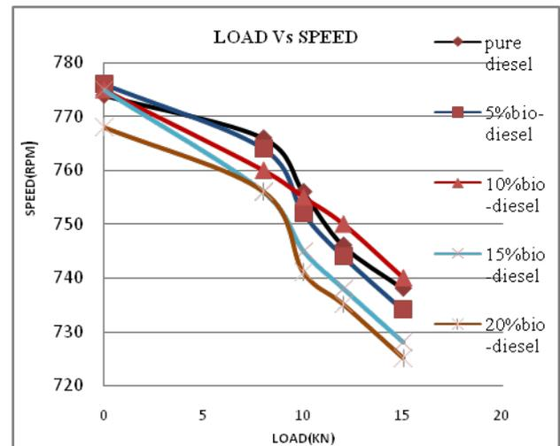
Fig. 7.1 Variation of speed with load for pure diesel and diesel blends with biodiesel
