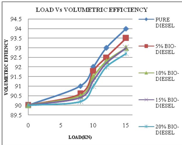
Fig. 7.3 Variation of volumetric efficiency with load for pure diesel and diesel blends with biodiesel
