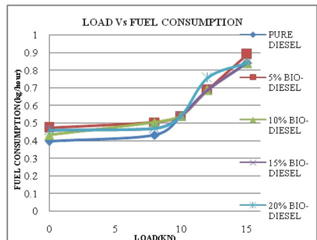
Fig. 7.2 Variation of fuel consumption with load for pure diesel and diesel blends with biodiesel
