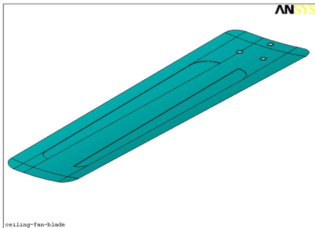
Fig. 2.1 CAD model of Ceiling Fan Blade
