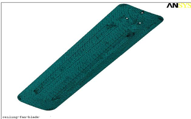
Fig. 2.2 Meshing of Ceiling Fan Blade
