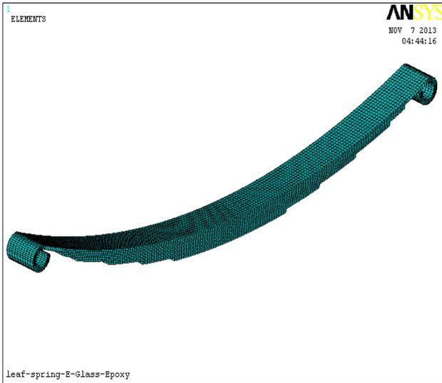
Fig. 4.1 Meshed view of leaf spring
