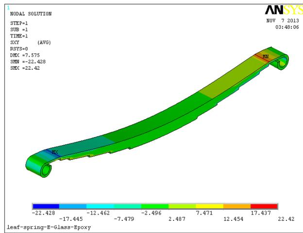
Fig. 5.6 Shear stress in XY direction (E Glass Epoxy)
