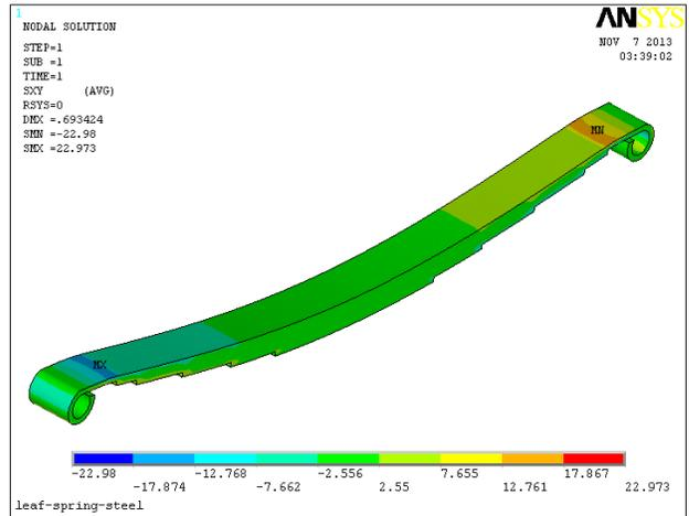
Fig. 5.5 Shear stress in XZ direction (Steel)
