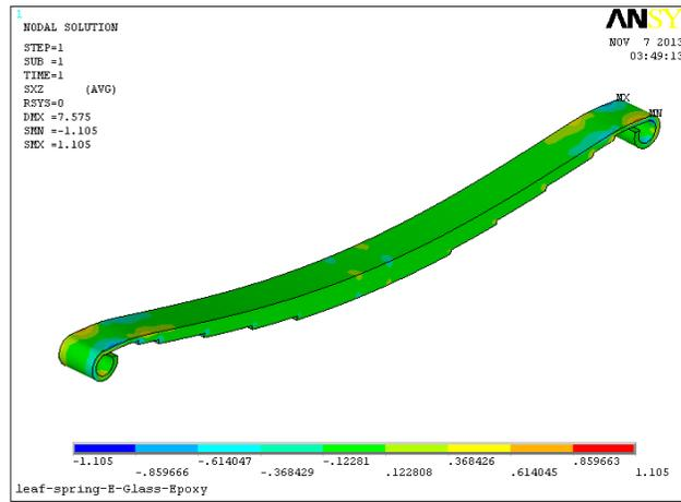
Fig. 5.7 Shear stress in XZ direction (E Glass Epoxy)
