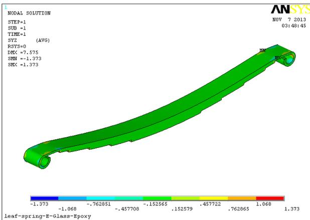
Fig. 5.9 Shear stress in YZ direction (E Glass Epoxy)
