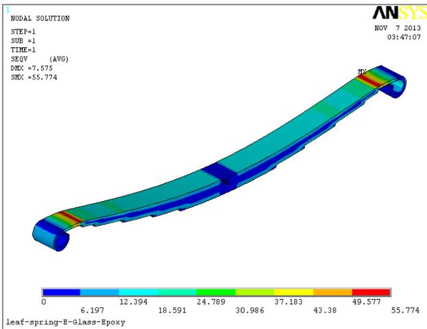
Fig. 5.3 Von moises stress in E Glass Epoxy
