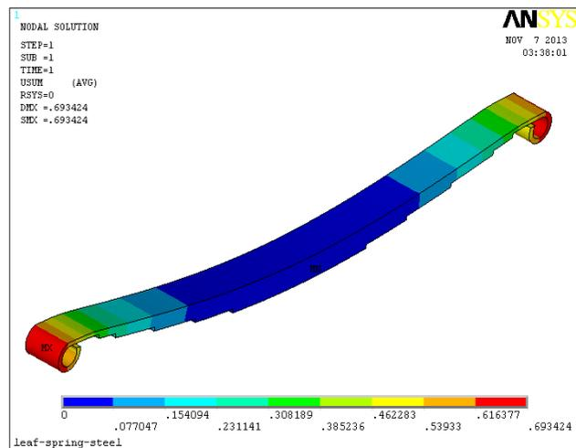
Fig. 5.1 Displacement diagram
