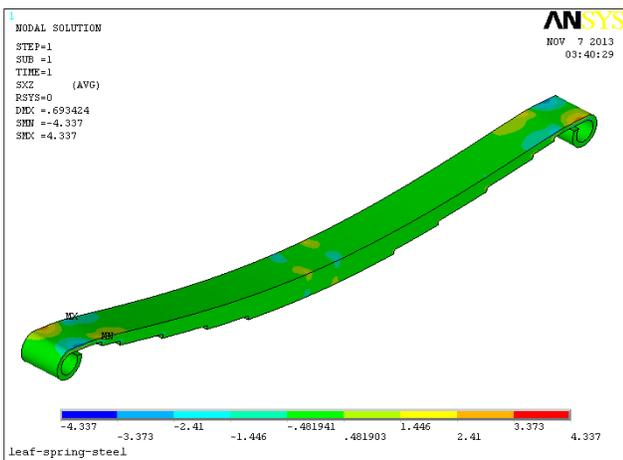
Fig. 5.4 Shear stress in XY direction ( Steel )
