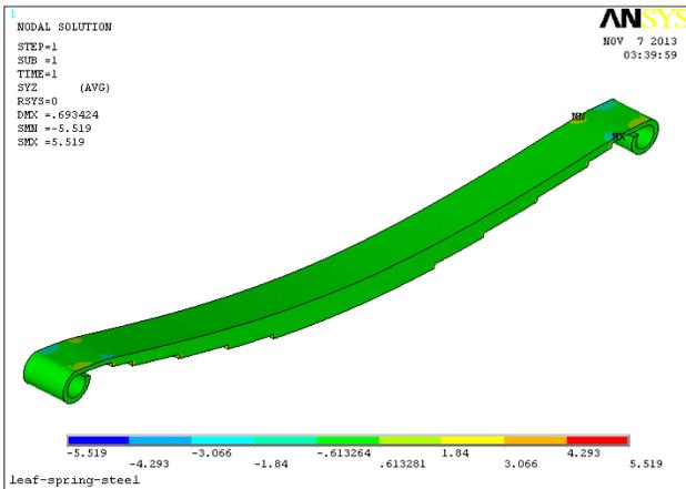
Fig. 5.8 Shear stress in YZ direction (Steel)
