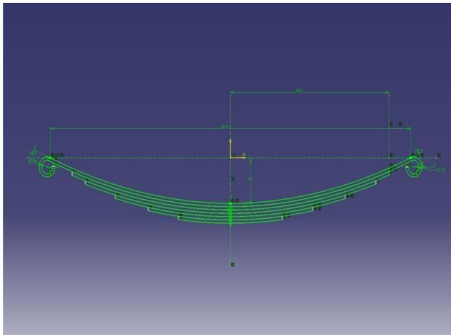
Fig. 4.2 Dimensioned view of leaf spring
