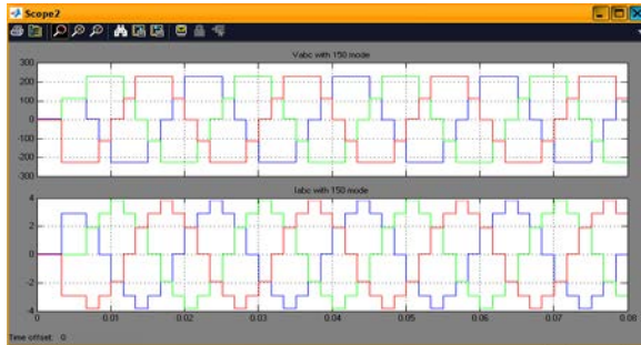
Fig.3.1 Three phase Load Current and Load Voltage waveform for inverter 150° mode of conduction without filter .
