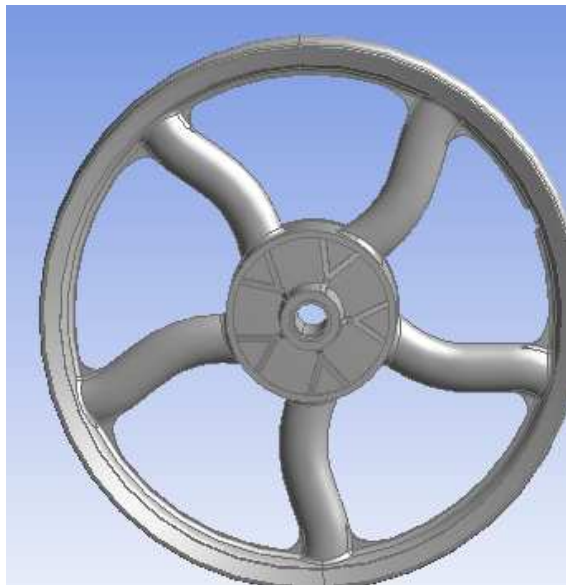
Fig 3.1 Design of alloy wheel using PEEK material
