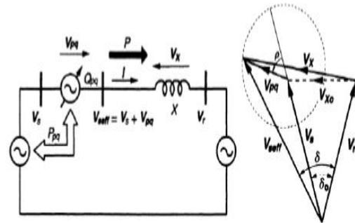
Fig 3.2 - Conceptual representation of Unified Power flow Controller
