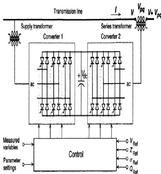
Fig 3.1 Unified power flow controller
