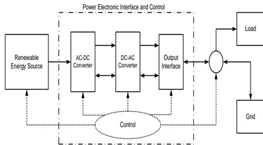
Fig.3.1- Generalized diagram of power electronic interface
