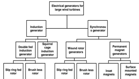
Fig.2.1- Classification of commonly used electric generators used in WECS
