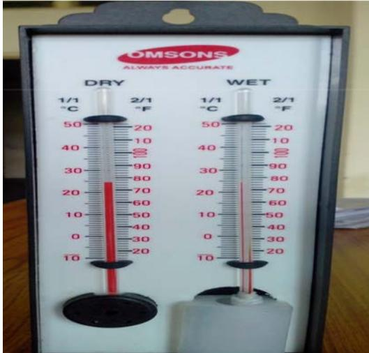
Fig3.3- DBT and WBT Thermometers.
