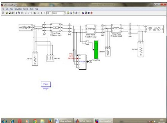
Fig. 3.3 - MATLAB Simulink Model of STATCOM
