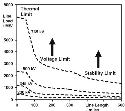
Fig.2.1- Operational Limits of transmission lines for different voltage levels.
