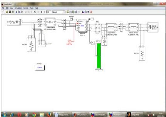
Fig. 3.2 - MATLAB Simulink Model of SSSC System
