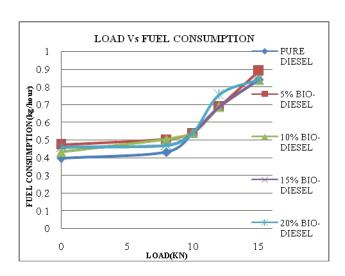
Fig. 7.2 Variation of fuel consumption with load for pure diesel and diesel blends with biodiesel
