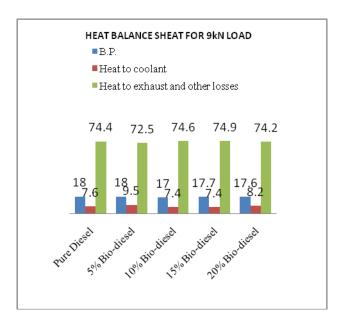
Fig. 7.6 Heat balance sheet for 9 kN Load
