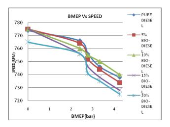
Fig. 7.4 Variation of speed with BMEP for pure diesel and diesel blends with biodiesel
