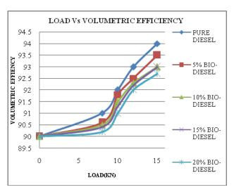
Fig. 7.3 Variation of volumetric efficiency with load for pure diesel and diesel blends with biodiesel
