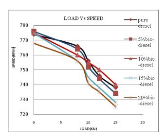
Fig. 7.1 Variation of speed with load for pure diesel and diesel blends with biodiesel
