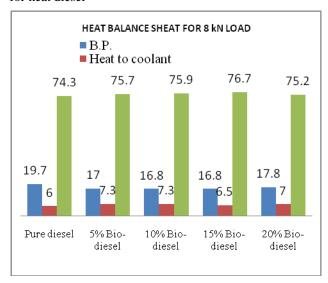
Fig. 7.5 Heat balance sheet for 8 kN Load
