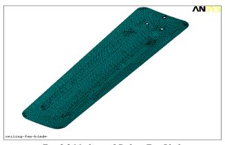
Fig. 2.2 Meshing of Ceiling Fan Blade
