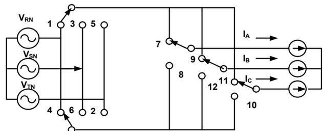
Fig.3.2 - Indirect matrix converter
