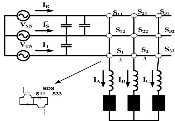
Fig.1.1- Basic matrix converter
